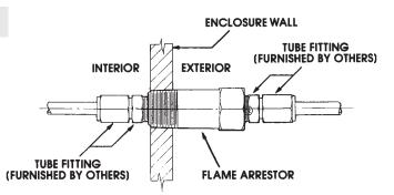
Exterior enclosure wall counter boring may be required to maintain  $\frac{1}{2}$  enclosure wall thickness for ease of field connections.
